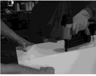
5) Pin-nail the three panels together into one unit. *See column cover instructions!*
