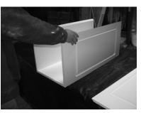
4) Assemble two panels to glued edges of panel from step 3.
